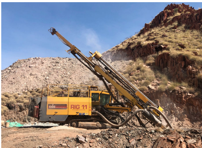
Above: An RC rig at Warrawoona infill drilling to upgrade indicated material into the measured category.
