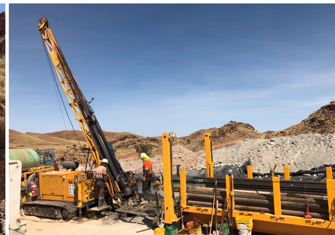
Above: A diamond rig drilling Klondyke deeps. Drilling RC pre-collars for the first 200m with diamond tails.
